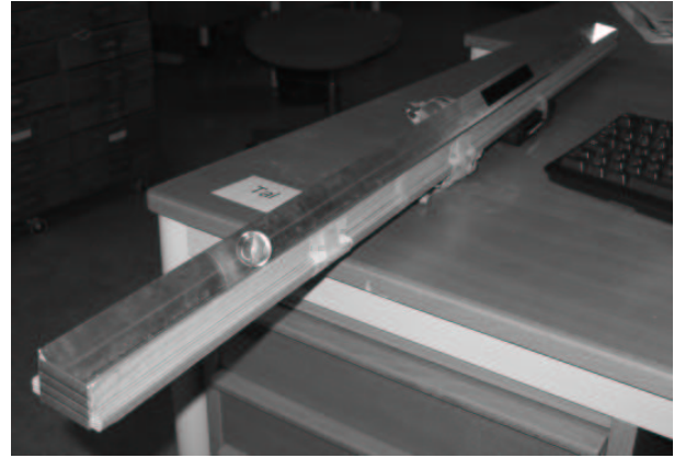
Fig. 4. The “rolling-track” with a glass marble rolling in its upper-face aluminium track.
