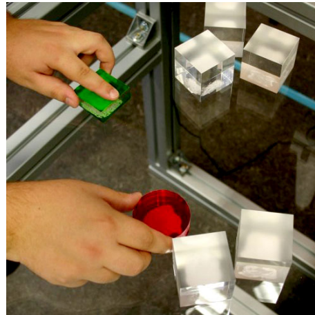
Figure 1: Tangible Interactive Sonification - showing bimanual interactions while interactively tuning the sonification of stock market data. The red object is the sonification object, which here acts as listener to data streams.
