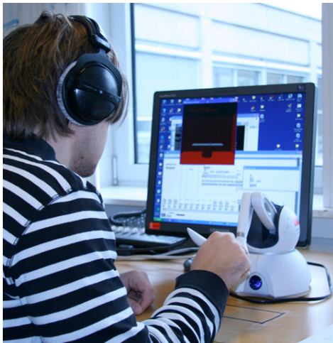
Figure 4. The experimental setup with a test subject placed in front of the Phantom® Omni™ haptic device.
